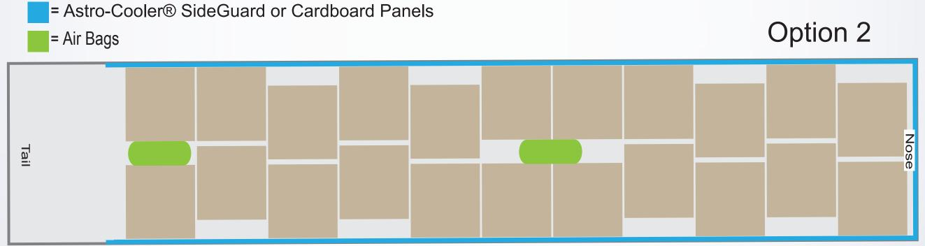
Intermodal Container Interior: L 630" x W 98" x H 106" ~ Pallets: 48" x 40" ~ if pallets are not utilized: Astro-Cooler® FloorGuard is available
