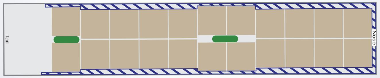
Intermodal Container Interior: L 630" x W 98" x H 106" ~ Pallets: 48" x 40" ~ if pallets are not utilized: Astro-Cooler® FloorGuard is available
